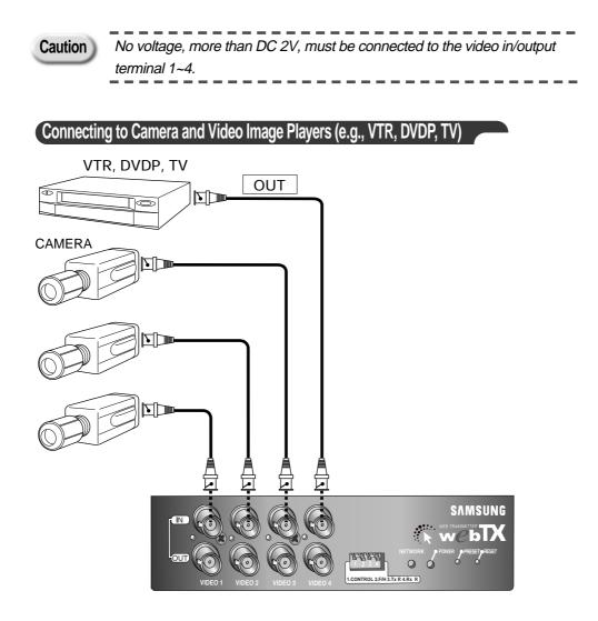
SNS-110 automatically detects NTSC/PAL and transmits it as image signal. Therefore, you may connect cameras and video image players (e.g., VTR, DVDP, etc.,) to video terminal 1~4.
